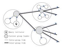
Fig. 3. A grouping demo of the unstructured P2P system. The dotted blue arrow illustrates the message flow of a search operation.
